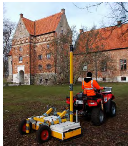
Fig. 1: MALÅ MIRA multichannel 3D GPR array (16channel, 450MHz version) with total station mast.
