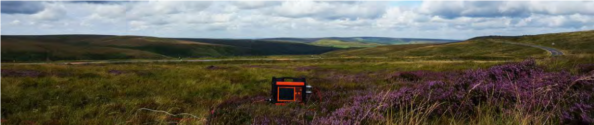
Fig. 3: ABEM Terraloc Pro seismograph mapping upland peat deposits.
