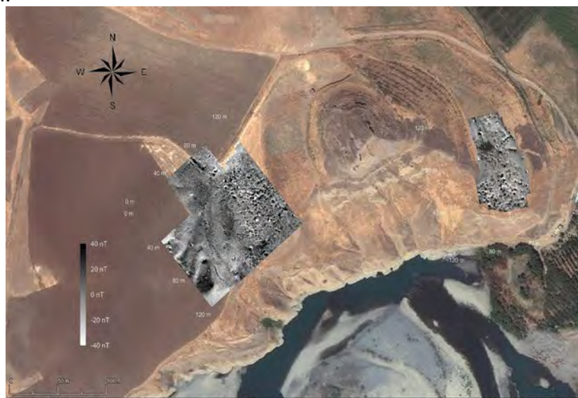
Fig. 2: Qalat-i Dinka. Magnetometer measurement of the survey area (ca. 120 × 120 m), on the slope of the fortification. Caesium total field magnetometer Scintrex, SMG-4 special in duo-sensor variometer configuration, total Earth's magnetic field at the Peshdar Plain 08/2015, 47.500 ±20 Nanotesla, sensitivity ± 10 Picotesla, sampling density 25 × 50 cm, interpolated to 25 × 25 cm, dynamics in 256 grey scales, 40 m grid, high-pass filter overlay.
