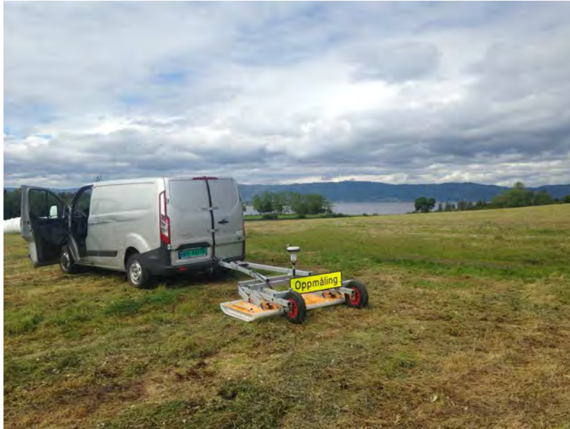
Fig. 2: High-resolution GPR conducted with a 3d-radar Mark IV GPR-system with a ground coupled antenna array.
