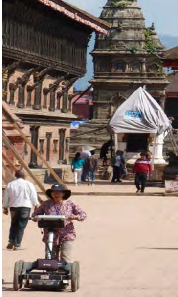
Fig. 2: GPR survey on Bhaktapur Durbar Square.
