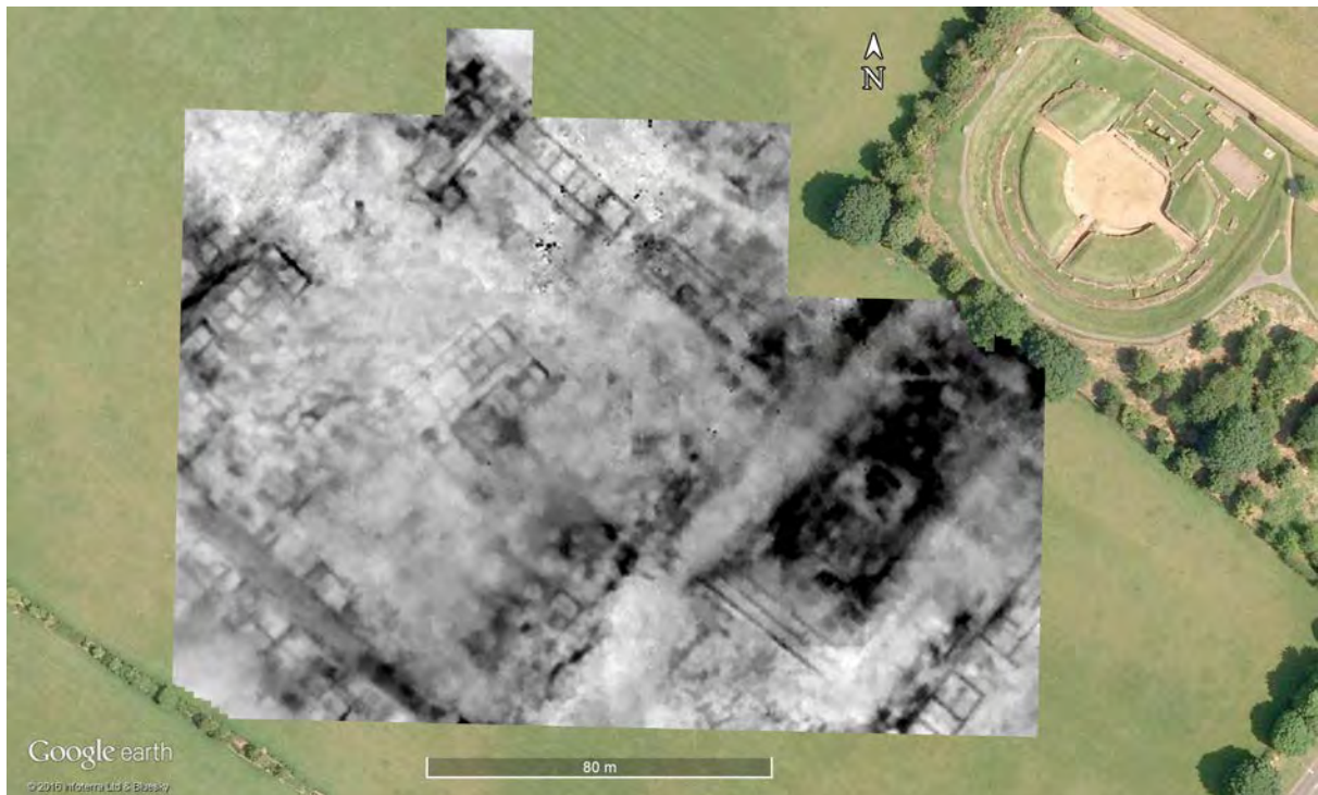
Fig. 4 The resistance survey (black as high resistance).
