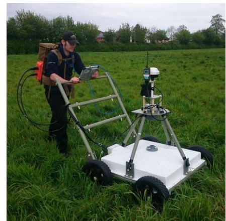
Figure 1: MetalMapper2x2 advanced Time Domain Electromagnetic Metal detector
