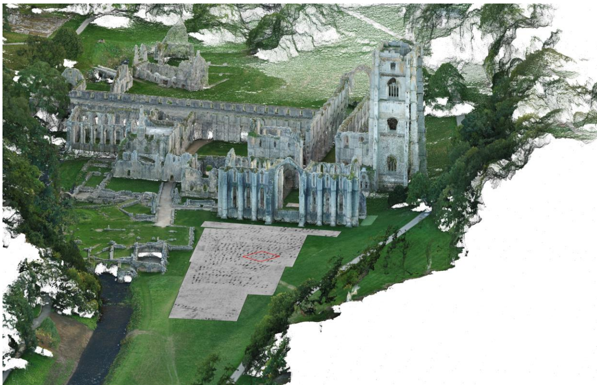
Figure 2: Location of excavation superimposed on GPR image and with point cloud derived from drone data
