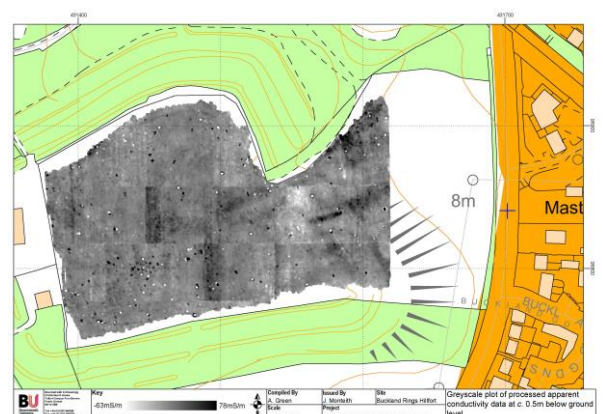
Figure 3: Conductivity ( EC_a ) survey of Buckland Rings Iron Age Hillfort showing the extent of the ploughed-out ramparts, modern paths, and several circular features.
