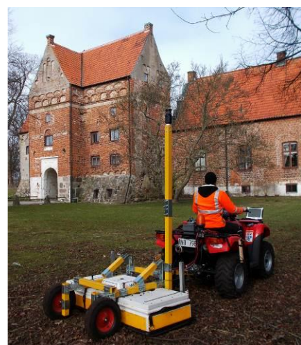
Figure 1: MALÅ MIRA multichannel 3D GPR array (16channel, 400MHz version).
