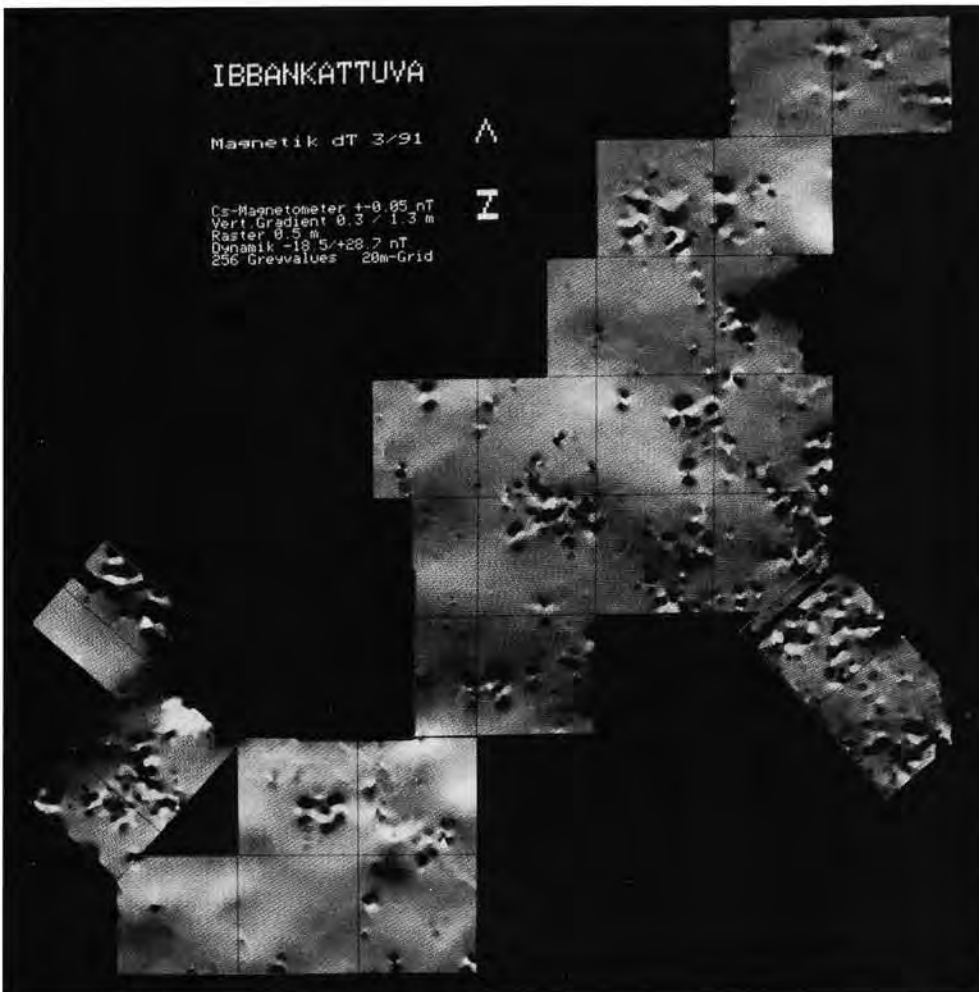
Fig. 3. Ibbankatuwa. Digital image of the magnetometer data of the surveyed area at Ibbankatuwa. Magnetogram in the digital image processing technique. Caesium magnetometer system from Varian/Scintrex, V101, Canada, sensitivity \pm 0.1 Nanotesla, gradiometer configuration, dynamics -10.0 to +15.0 Nanotesla in 256 greyscales, sampling rate 0.5 meter, grid 20 x 20 meter
