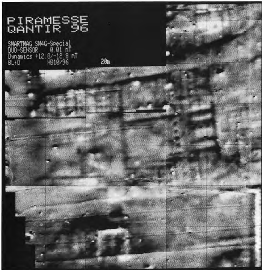
Fig. 3a. Qantir-Piramesses 1996. Magnetogram as digital image with 256 gray-scales. Raster 0.5/0.25 m, dynamics -12.8+12.8 nT (black/white), square mean, edge matching and desloping, 20 m grid
