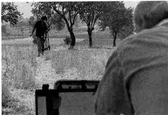
Fig. 3. Troy 1992. Magnetic prospecting in the lower city of Troy in 1992 using the caesium magnetometer Scintrex V101 in the variometer mode; the base sensor is fixed to the middle tree in the background
