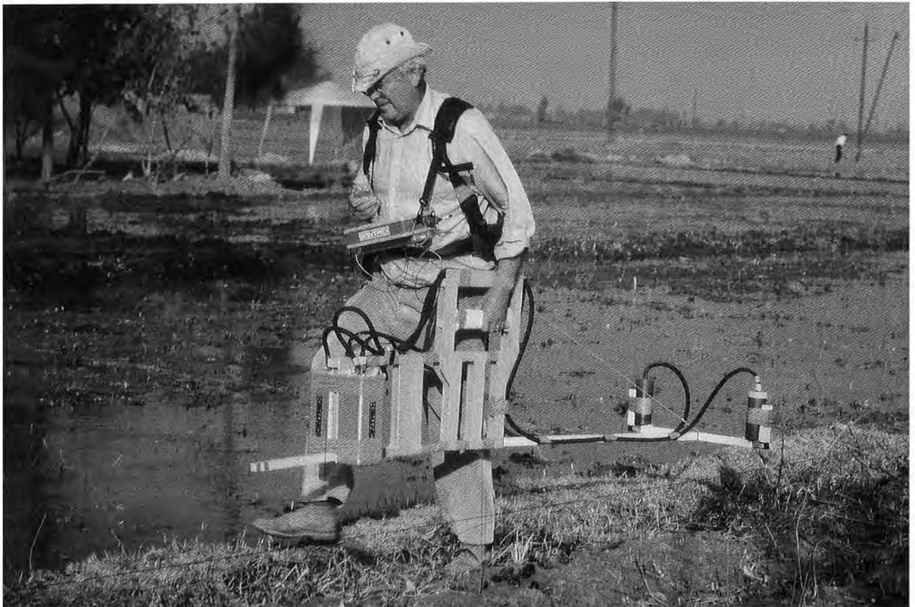
Fig. 2. Caesium Magnetometer Scintrex SM4G-Special with duo-sensor configuration and manual distance triggering every 5.0 m, sensitivity 10 pT (picotesla) at a cycle of 0.1 sec (Photo by J. Fassbinder)
