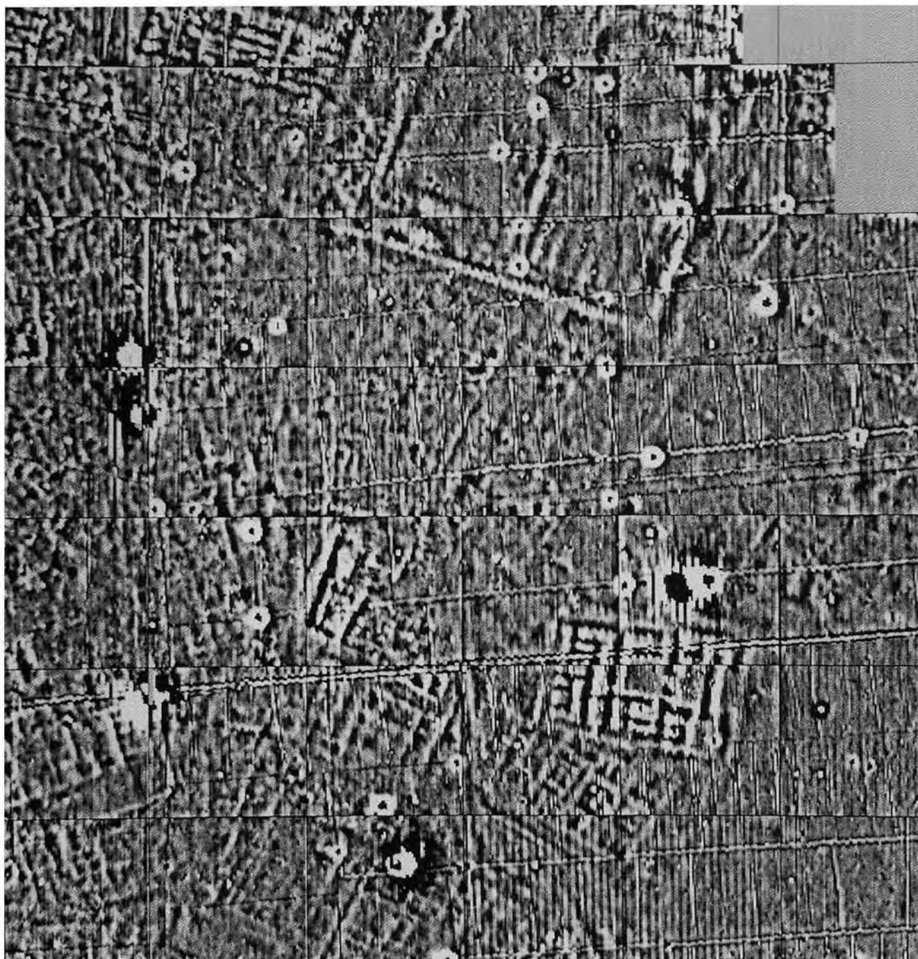
Fig. 5. Qantir-Piramesses East 1997/1998. Magnetogram of the same data as fig. 4, but highpass filtered data 10 x 5 pixel, technical data see Fig. 3a, 3b
