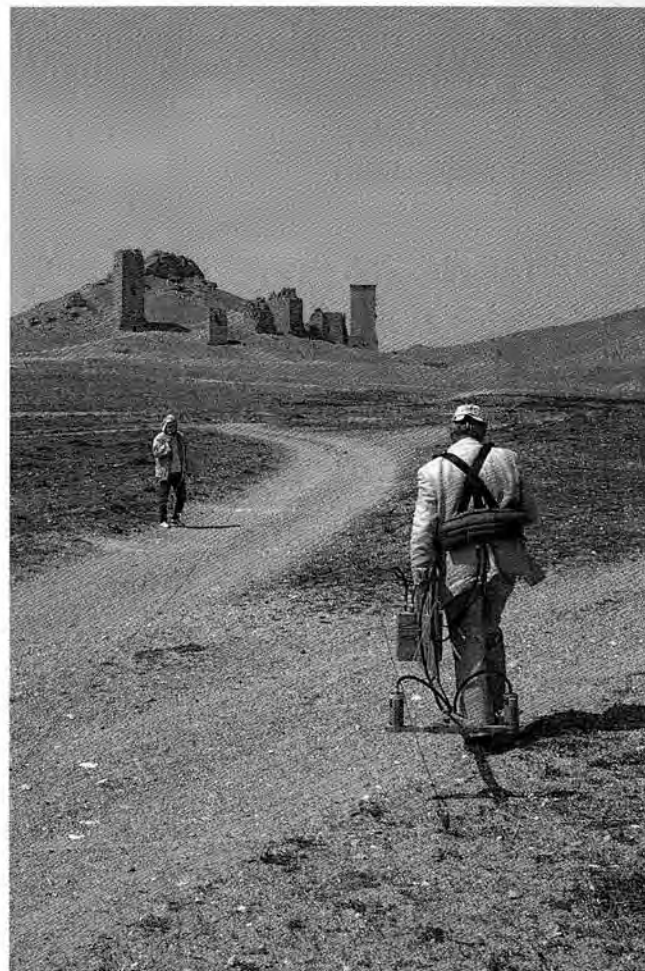
Fig. 2a, b. Palmyra 1997. Caesium magnetometer Scintrex Smartmag SM4G-Special with duo-sensor configuration for prospecting the Hellenistic city south of the wadi
