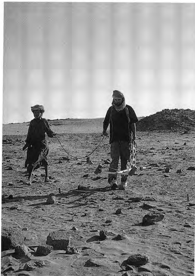
Fig. 1. Hagar Yahirr 11/1995. Caesium magnetometer CS2/MEP720 with duo-sensor configuration operated by J. Fassbinder
