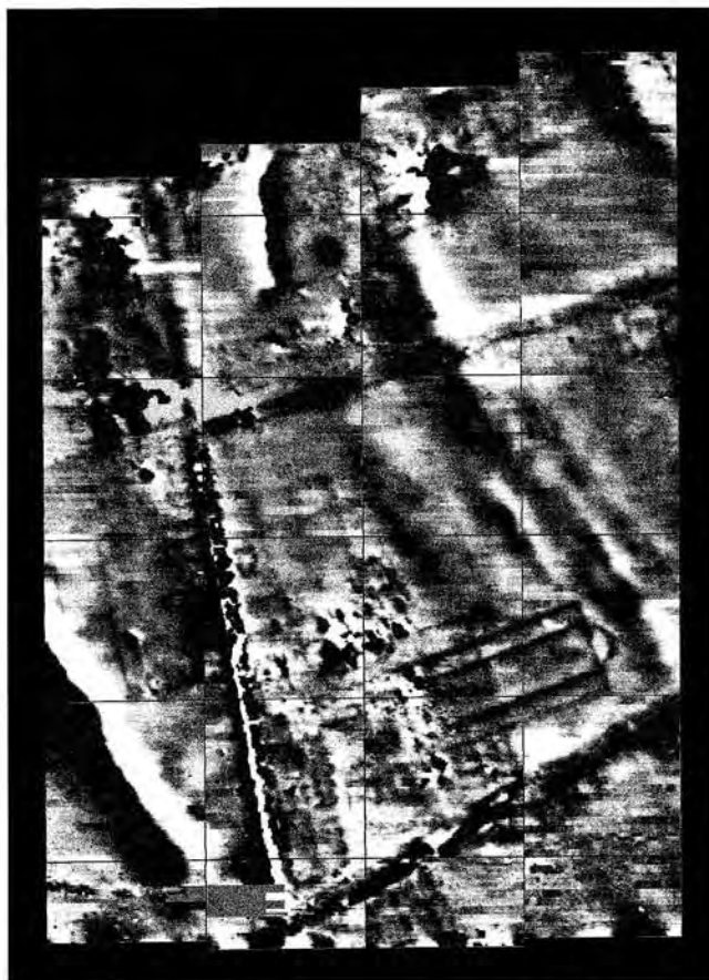
Fig. 6. Ostia Antica 1996 Magnetogram (detail with the basilica of Constantinus I.) in greyscaling, dynamics -50.00/+50.00 nT in 256 greyscale (white/black), sensitivity \pm 10 pT, raster after resampling 0.5/0.25 m, 1 Hz bandpass-filtering, reduction on 40 m line means, 40 m grid, Mag Nr. OS96-A
