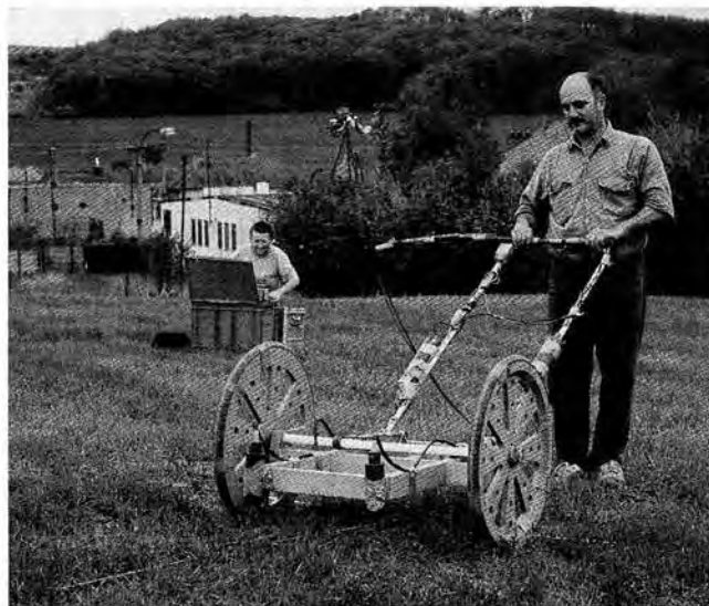
Fig. 2. Magnetic prospection with a Scintrex CS2 caesium magnetometer with the duo sensor configuration
