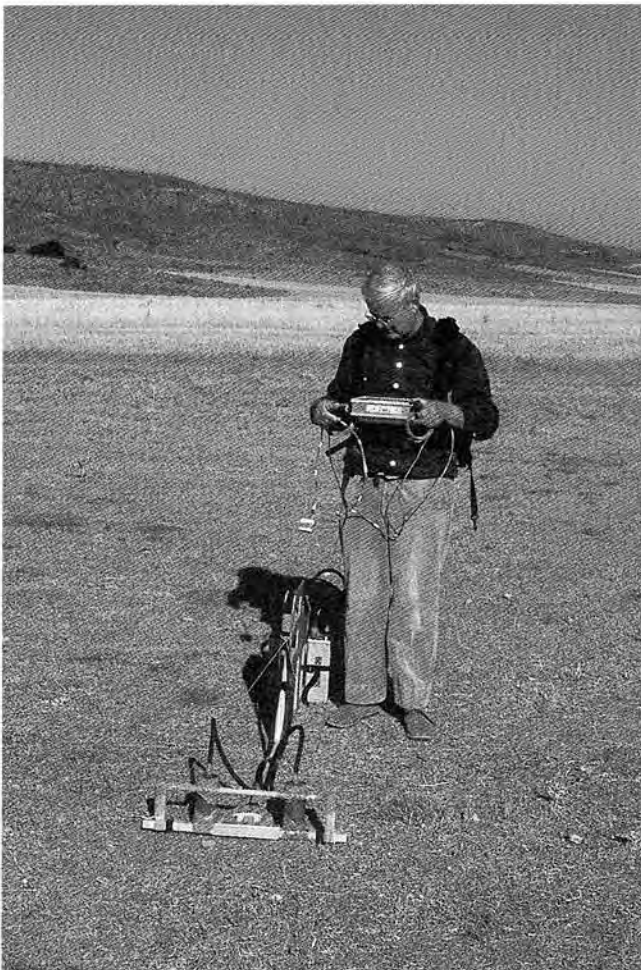
Fig. 1a. Ambrona-La Lampara 1996. Caesium magnetometry using Scintrex SMARTMAG SM4G-Special with duo-sensor configuration
