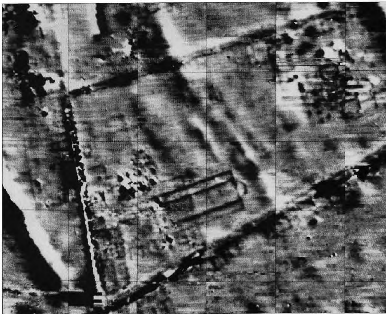
Fig. 4. Ostia-Antica 1996. Detail of the magnetogram of regio V with the newly discovered basilica of Constantinus I., the Great, clearly visible in the corner near the gate of the Via del Sabazeo and the city wall to the south. Caesium magnetometry SM4G-Special in quadro-sensor configuration, sensitivity 10 pT (= 0.01 nT Nanotesla), dynamics -50.0 /+ 50.0 nT in 256 grayscales (white/black), raster after resampling 0.25/0.5 m, 1 Hz bandpass filter, reduction of the diurnal geomagnetic variation by line-mean value, 40 m grid
