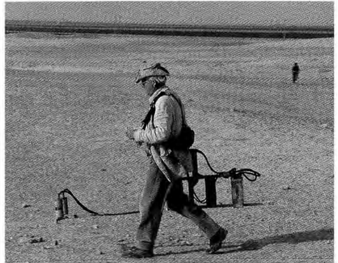
Fig. 2a, b. Duo-sensor on wheels with CS2/MEP720 system (application at Seehof, Photo J. W. E. Fassbinder) and one man carried SMARTMAG SM4G-Special (H. Becker in Resafa 1999, first use by H. Becker at Monte da Ponte in 1995)
