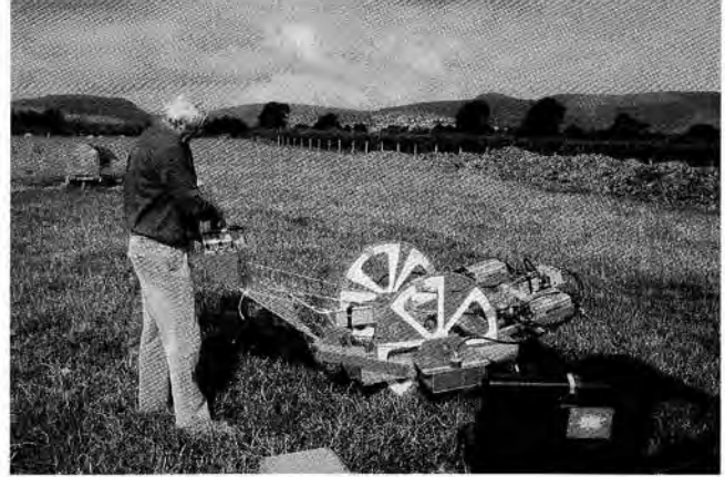
Fig. 1. "Magneto-Scanner" in Hindwell 1998; four caesium magnetometers Scintrex SMARTMAG SM4G-Special with quadrosensor configuration, two gradiometer consoles-data loggers, power supply (4 batteries 12 V/6 Ah) and automatic distance trigger mounted on a nonmagnetic chariot, total weight about 60 kg), type I/1996
